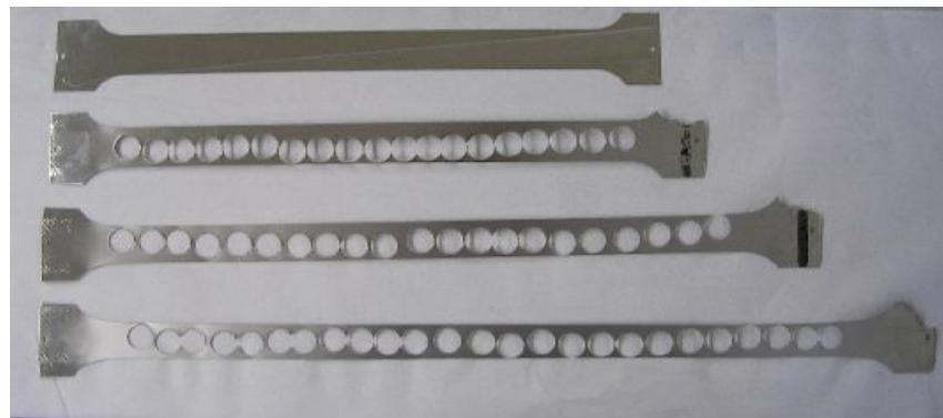
⇒ Disks stamped from strained samples to be used in electrochemical characterization.
