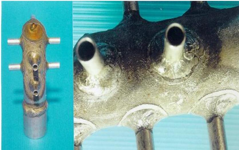
Example: Several secondary tubes are welded on a main tube. No post welding treatment was performed. Welds were then sensitised to intergranular corrosion, due to intergranular precipitation of chromium carbides in the heat affected zones.
